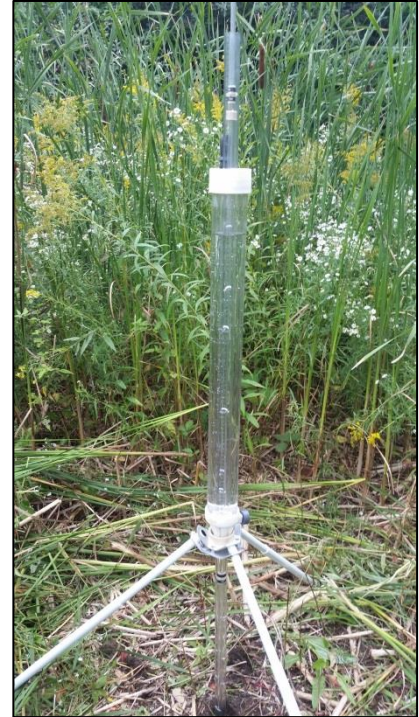
Figure 9.2: In-situ infiltration testing via Guelph Permeameter.
