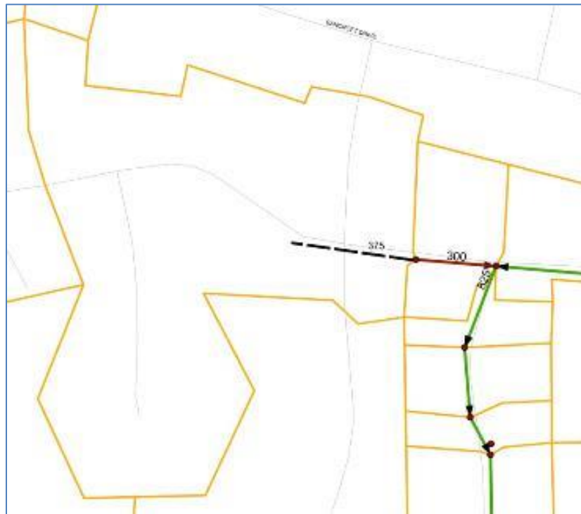
Figure 3.30: Connectivity with Pipes < 600 mm Diameter
