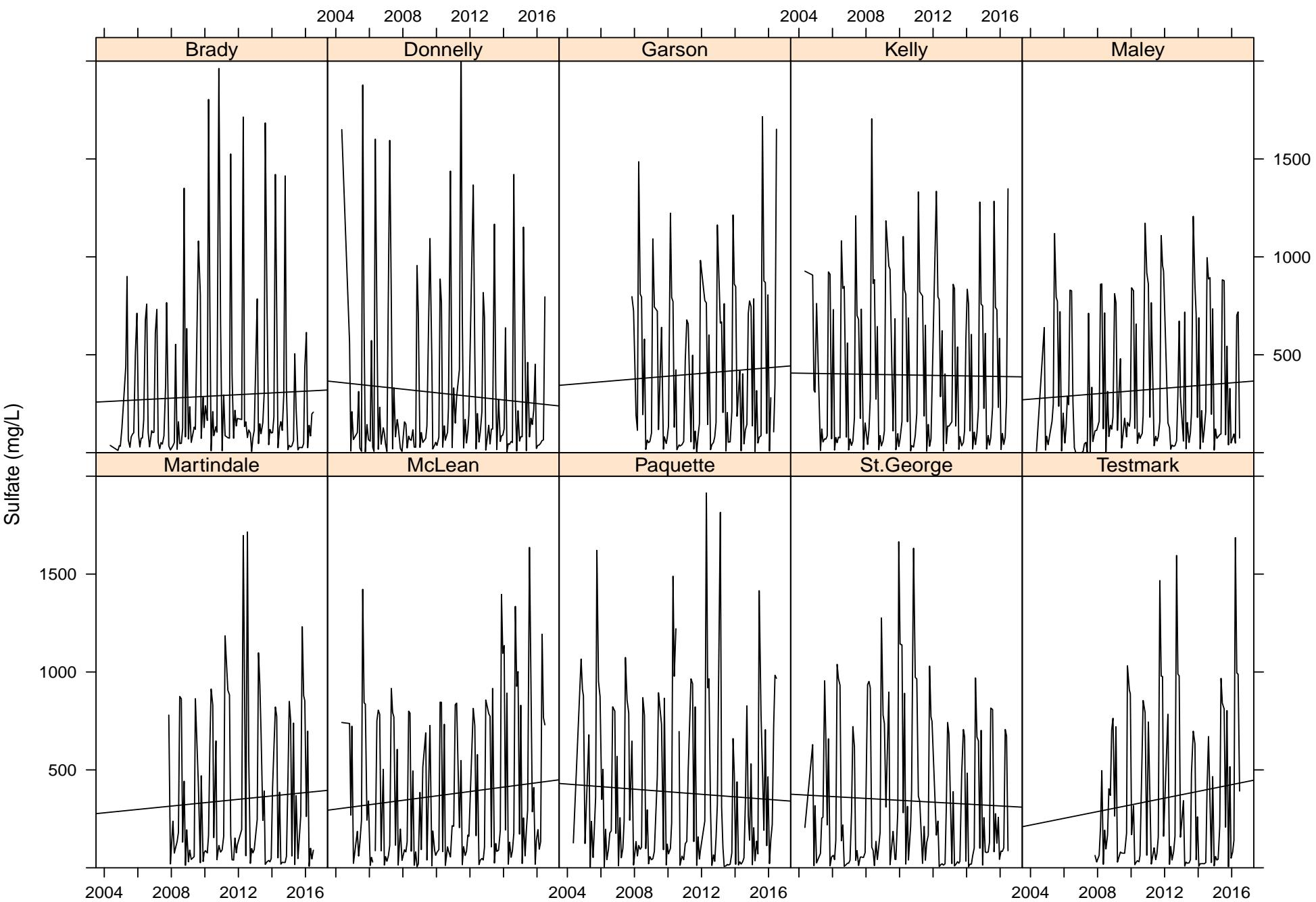
**Figure D24: Temporal Trends in Sulfate Concentrations within Junction Creek**
