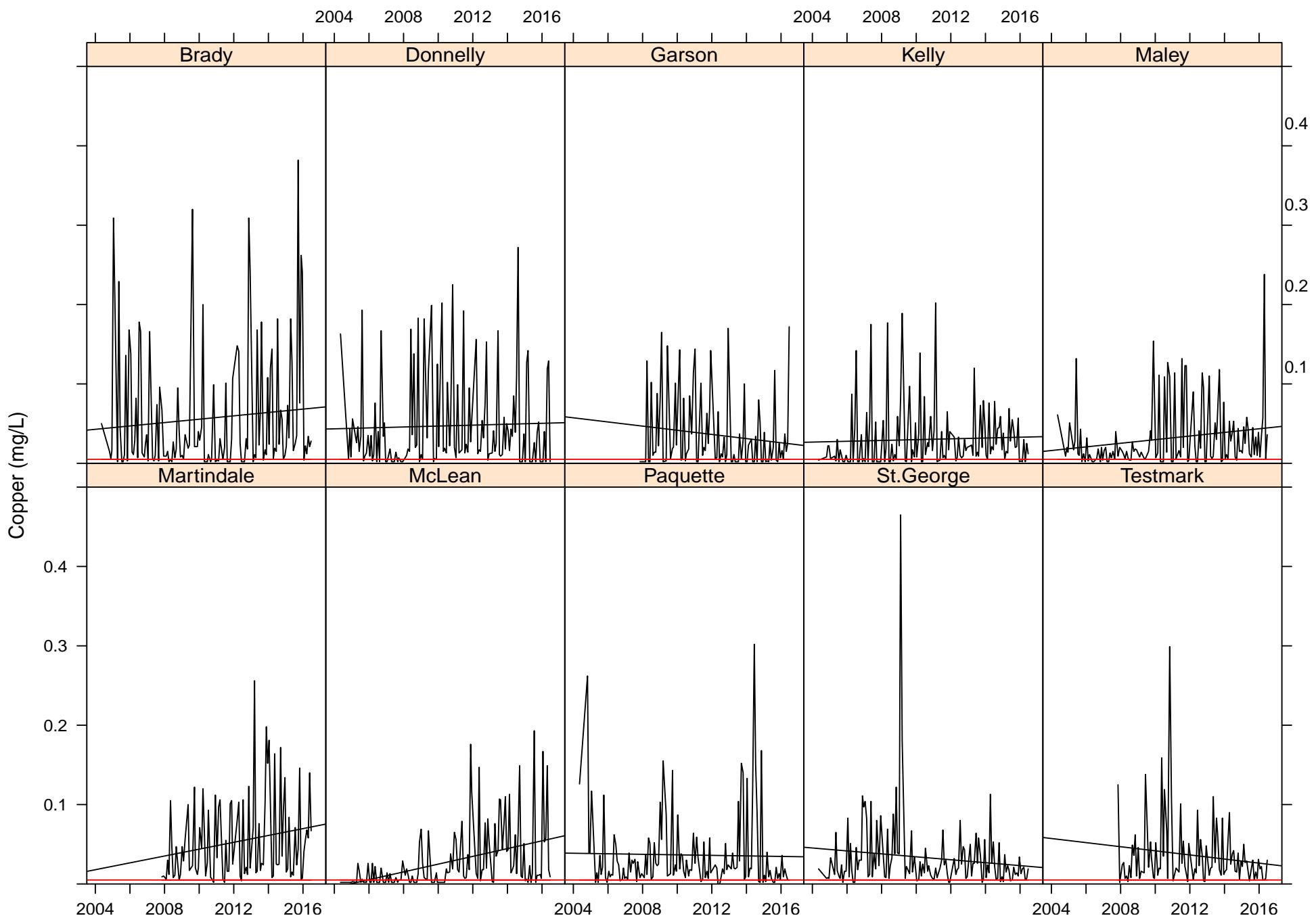
**Figure D8: Temporal Trends in Copper Concentrations within Junction Creek**
