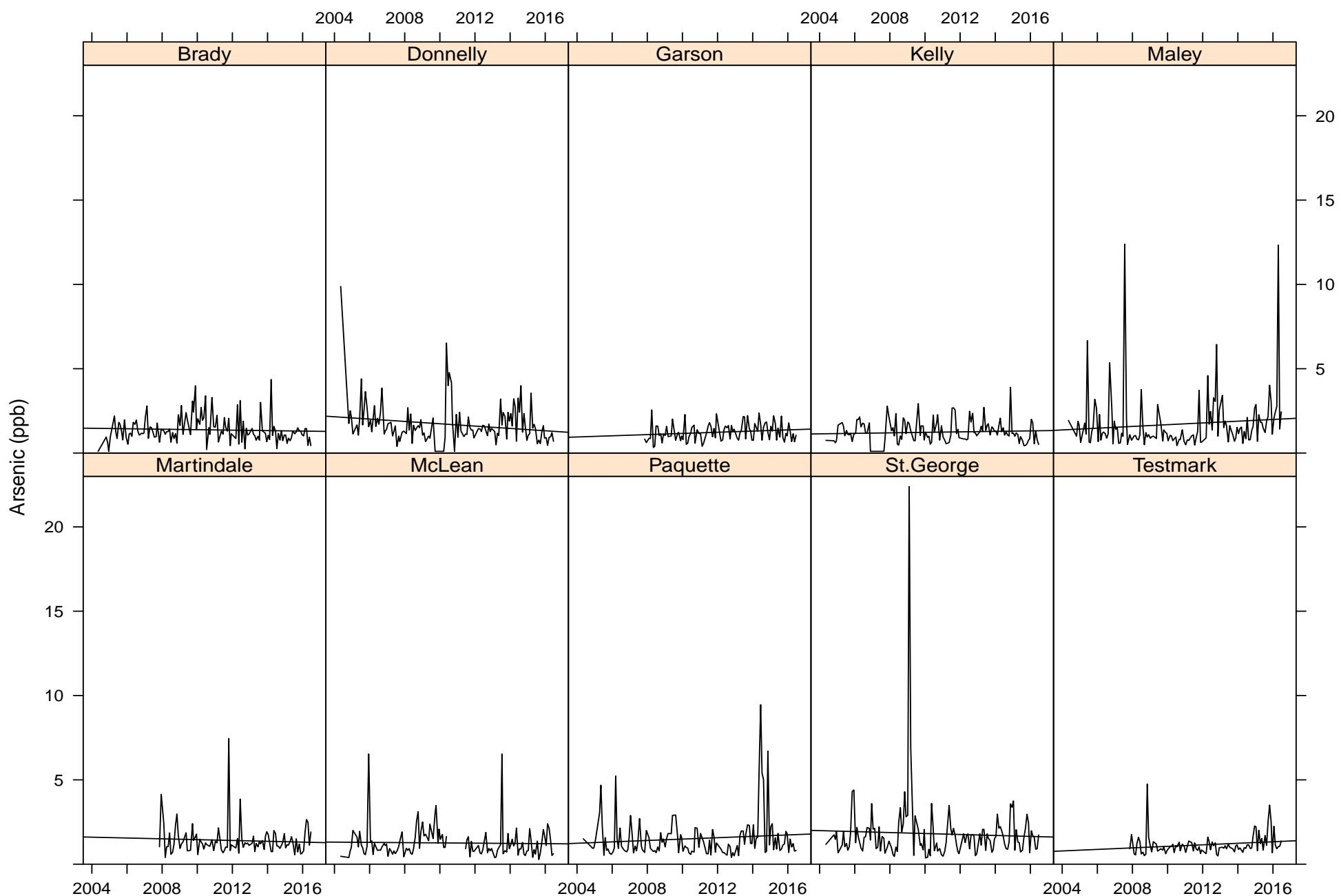
**Figure D4: Temporal Trends in Arsenic Concentrations within Junction Creek**
