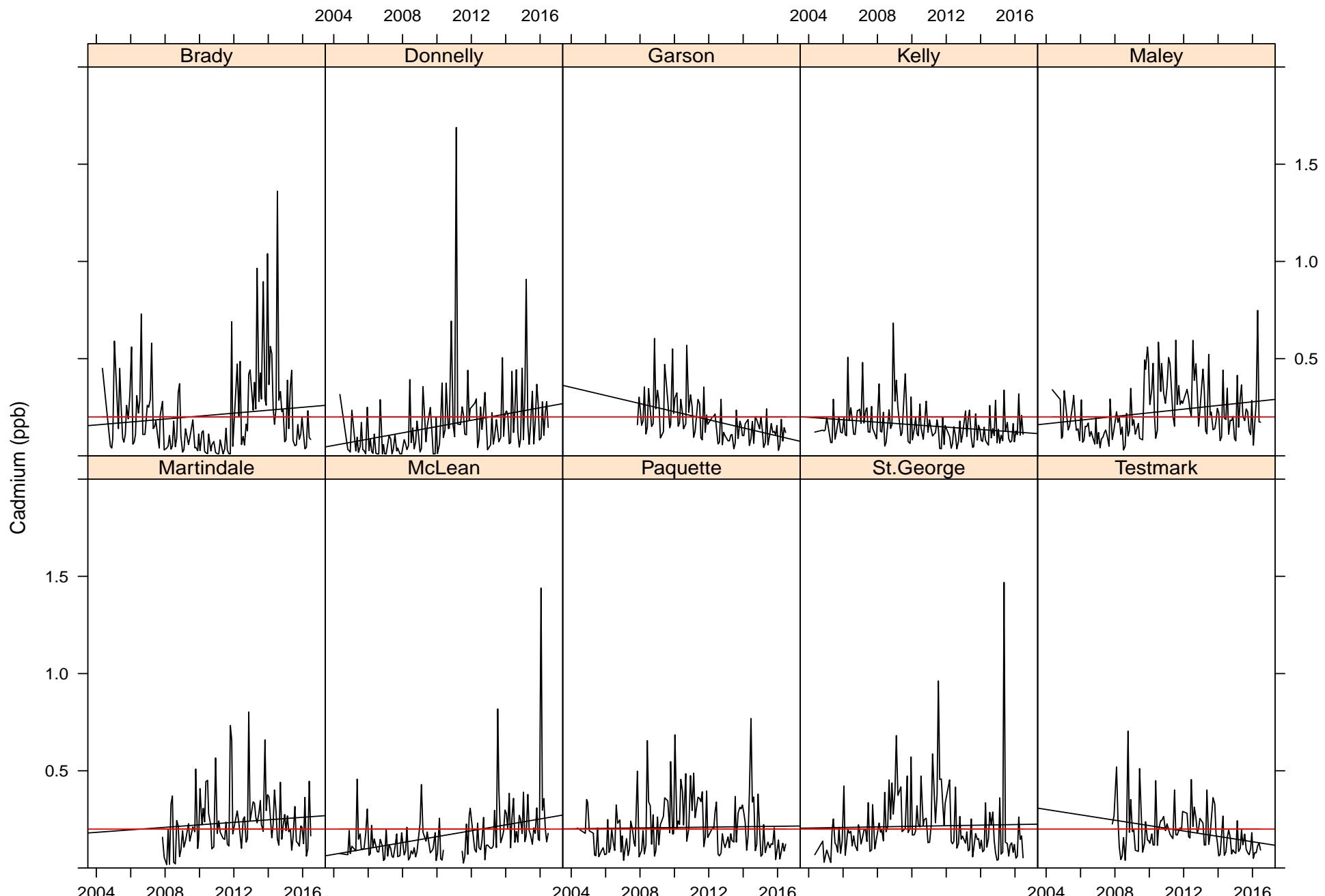
**Figure D6: Temporal Trends in Cadmium Concentrations within Junction Creek**
