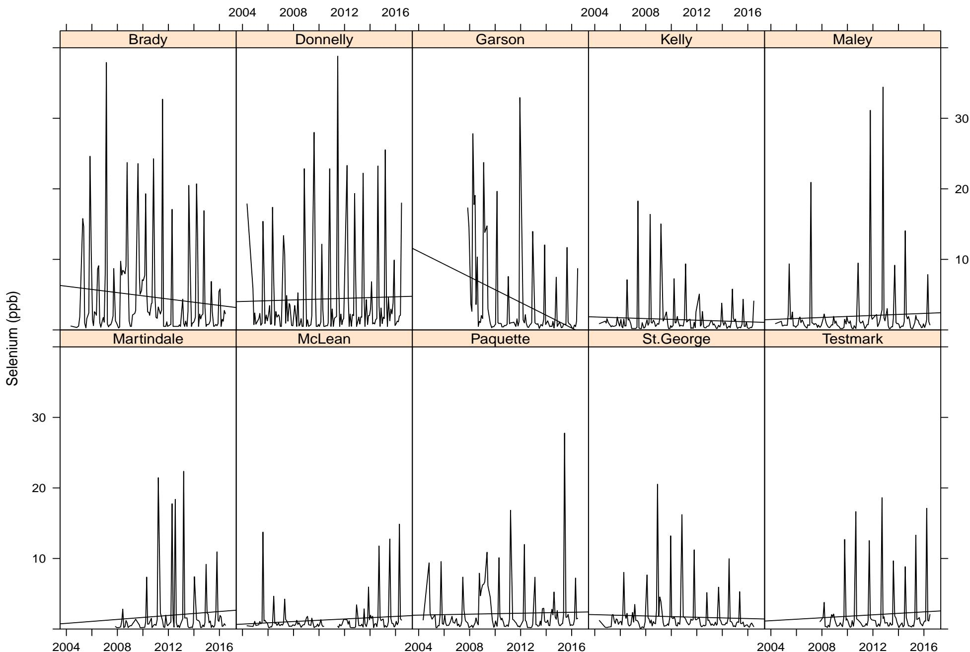
**Figure D23: Temporal Trends in Selenium Concentrations within Junction Creek**
