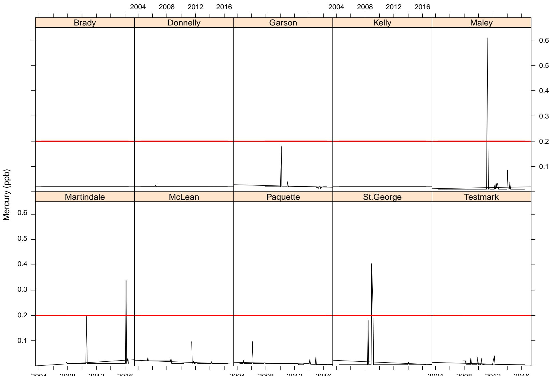
**Figure D12: Temporal Trends in Mercury Concentrations within Junction Creek**
