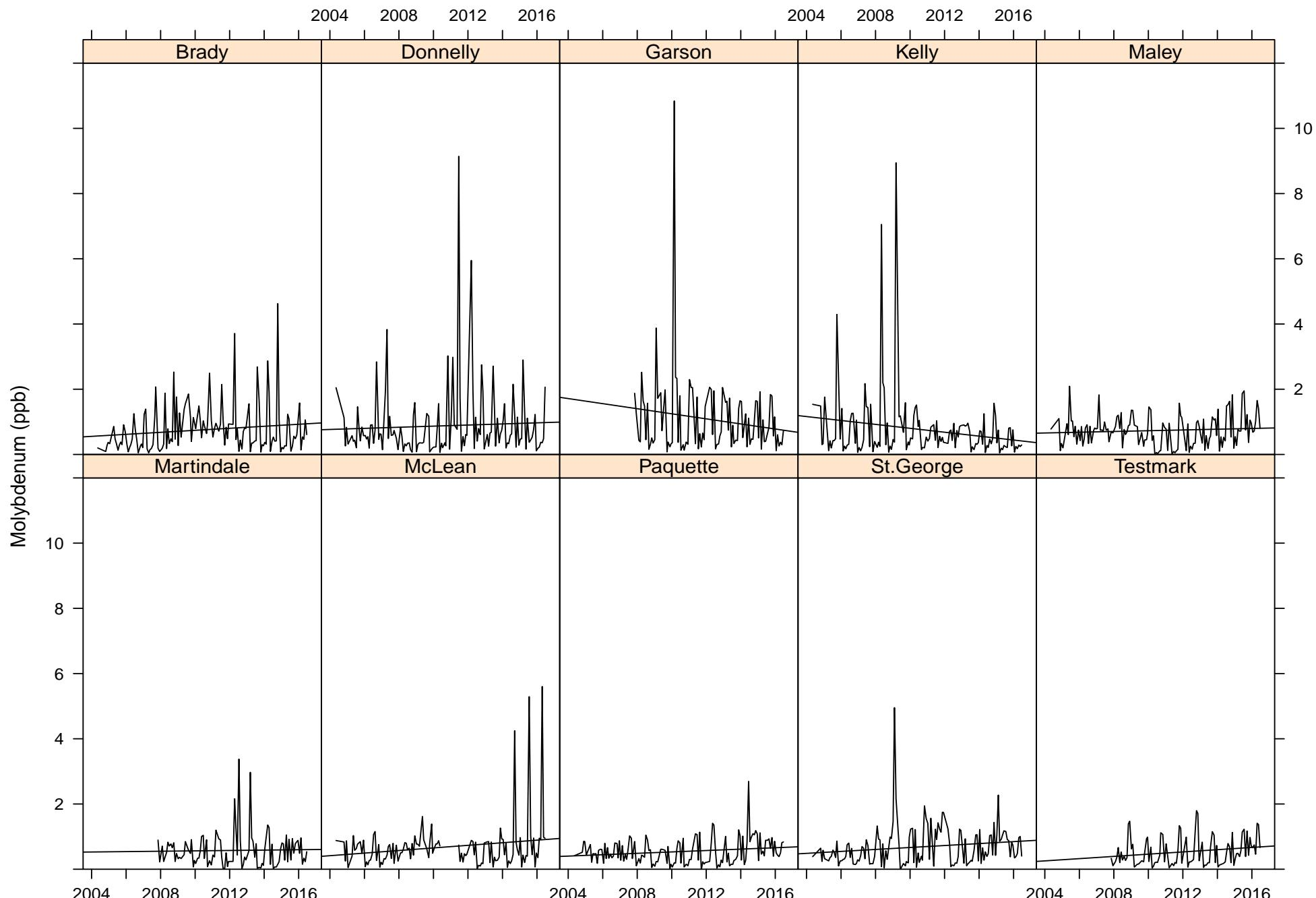
**Figure D16: Temporal Trends in Molybdenum Concentrations within Junction Creek**
