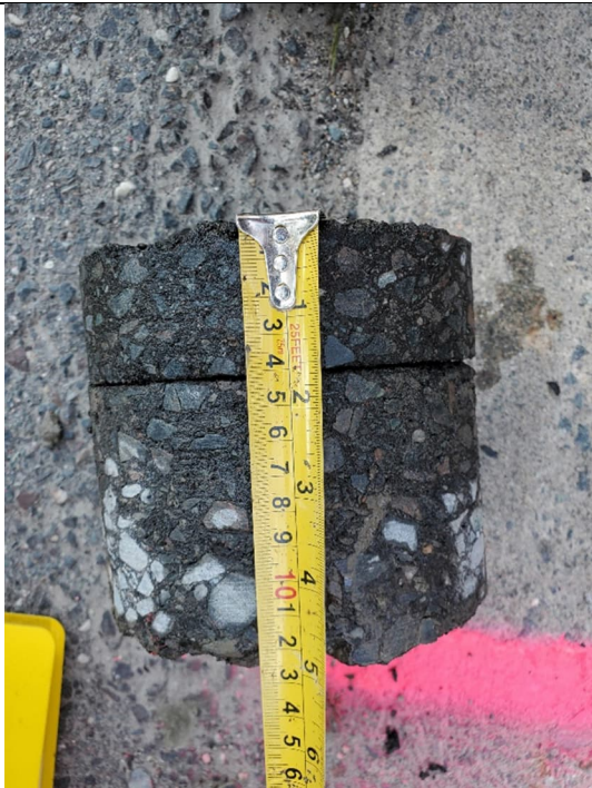
Photo 6: Additional Set 1, Core A1B, broken into 2 pieces.
