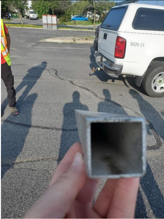
Photo 1: 3 m straight edge, used for level check.
