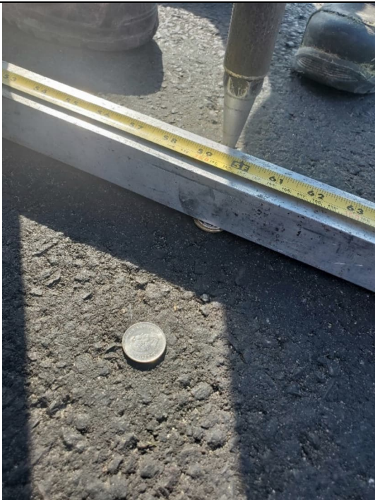
Photo 3: Survey Point 2, mid-lane 3 mm gap
