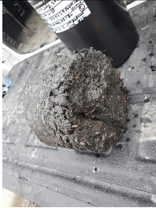
Photo 6: Core 11C with uneven bottom edge.
