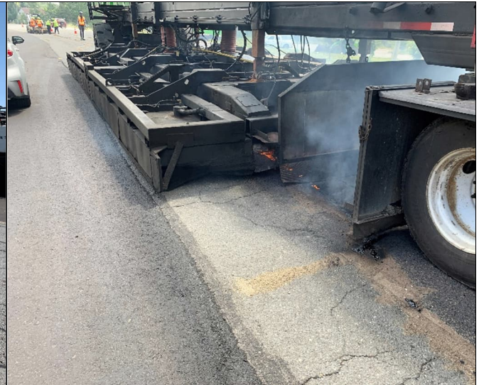
Photo 2: Open flame was observed in contact with the road surface.
