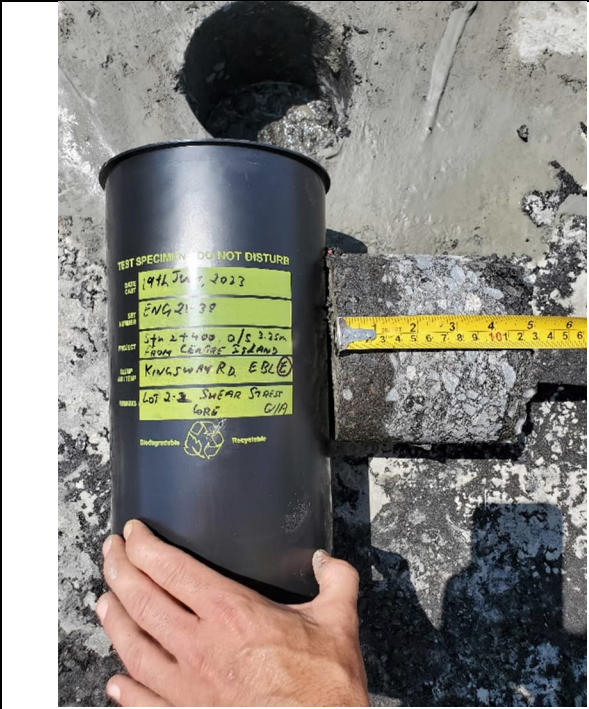
Photo 3: Core 3E next to its mould. Line between asphalt and underlying material is distinct.
