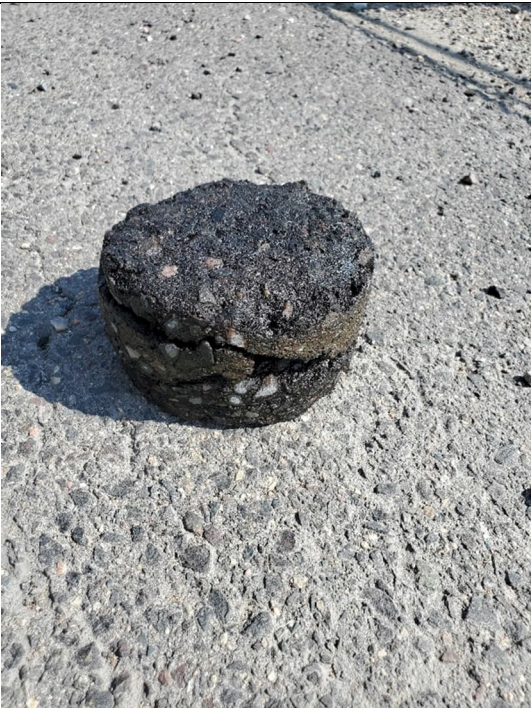
Photo 7: Additional Set 2, Core A2A, broken into 3 pieces.
