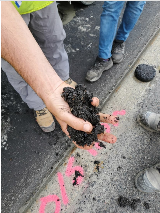
Photo 2: Wet, malleable asphalt/underlying material from the 5 th set of cores.
