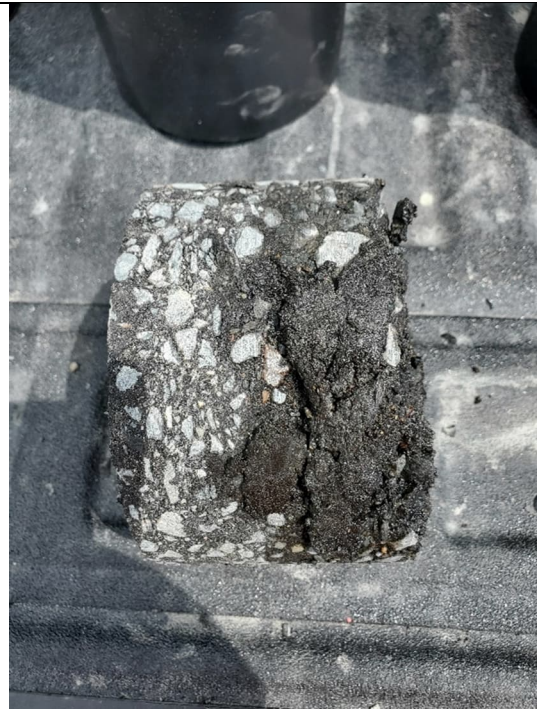
Photo 2: Core 17B (3-6, Q/C) with rubber stuck to outside of core sample.
