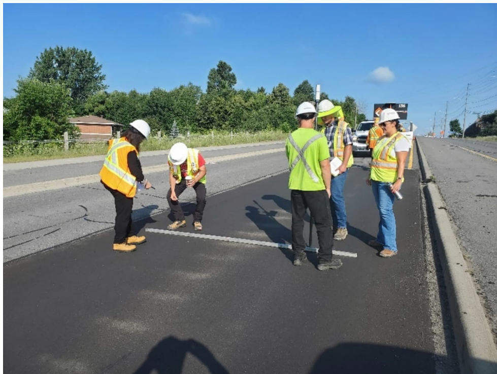
Photo 2: Surface Smoothness Testing with a 3 m Long Straight Edge
