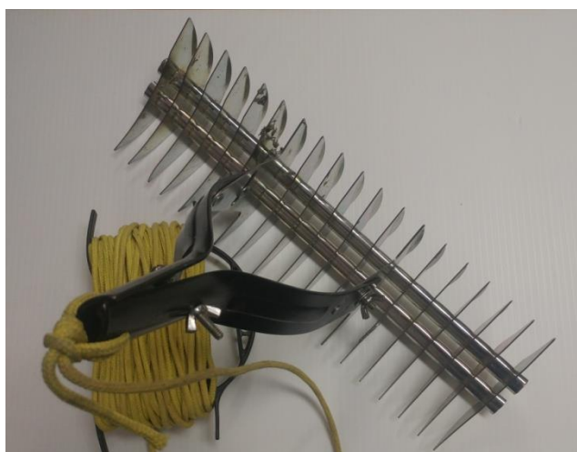
Figure 1. City of Greater Sudbury modified thatching rake used for aquatic vegetation sampling.
