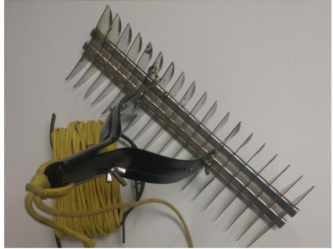
Figure 3. Modified Thatching Rake Used by the City of Greater Sudbury for Aquatic Vegetation Sampling
