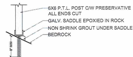
TYPICAL FOOTING DETAIL
