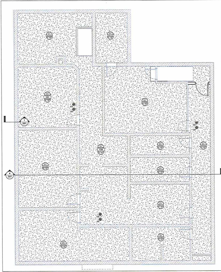
BASEMENT FLOOR REFLECTED CEILING PLAN 1/4" = 1'-0"
