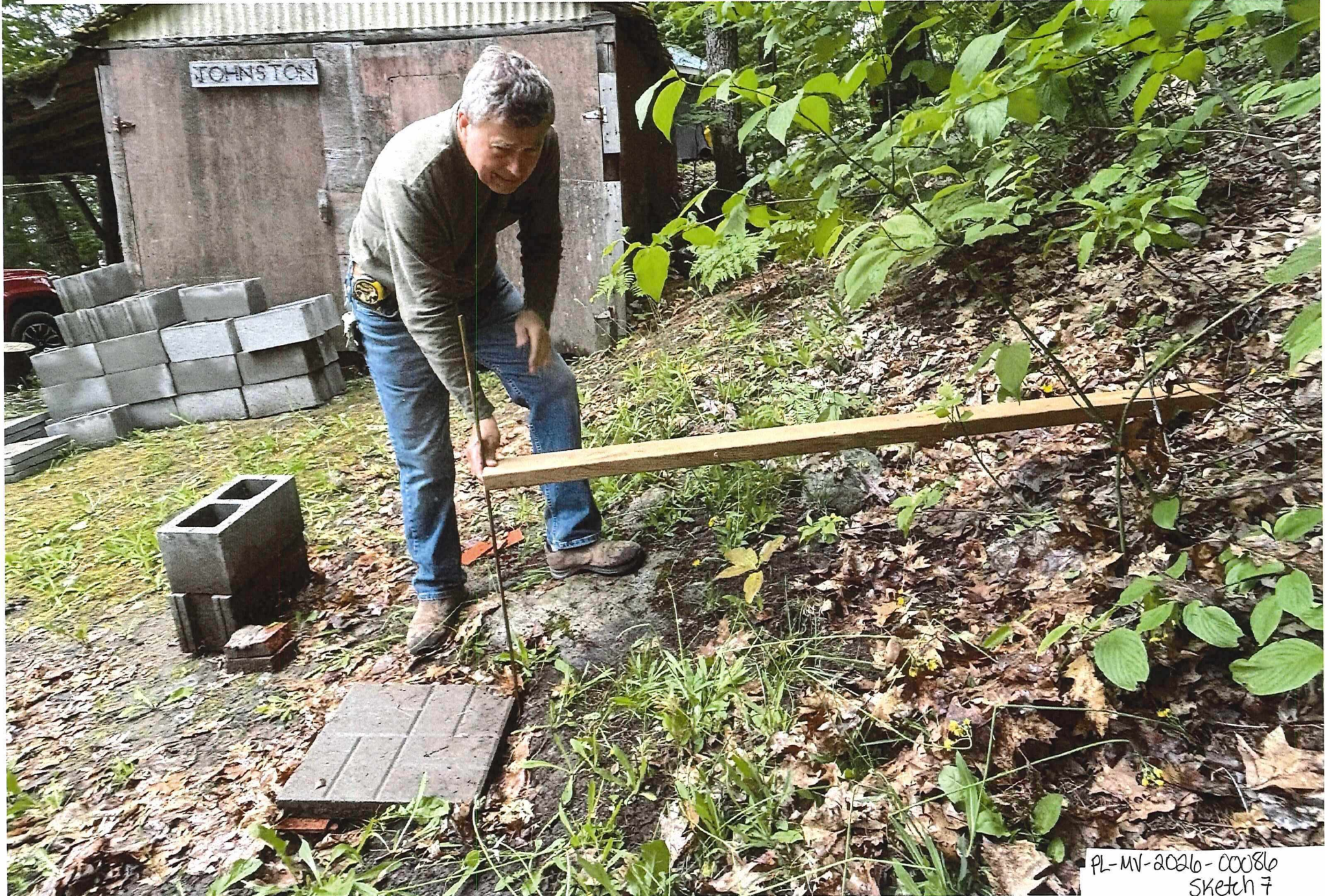
Picture 5: Pictures shows the west-facing view of the slope. We took a rough measurement 2m further north up the hill from the current placement, and took a visual of approximately how much higher the bunkie would be at that distance up the hill. You can see from this photo that even to bring the bunkie to a distance of 29m from the high water mark, would mean we would need to bring the height of the bunkie at the south corners to approximately .6m higher off the ground, or 1.2m height in total.
