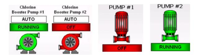
The following is an example pop-up screen providing typical SCADA control functionality for booster pumps (where available):
