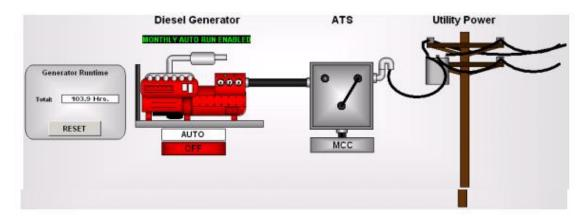
The next figure shows a pop-up screen which provides the interface for typical SCADA control of the emergency diesel generators (where available):
