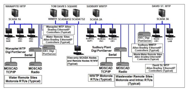
The City of Greater Sudbury Network is based on single mode fibre. Within facilities, the fibre network is owned by the City.
