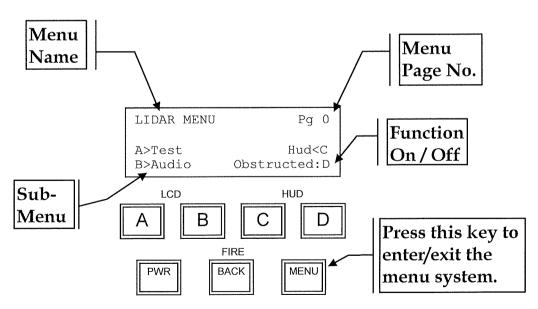
For each menu choice, on the outside left or right edge of the LCD is the letter matching the key to be pressed to activate the option. Between each key letter and its corresponding description is a symbol. The meanings of the symbols are as follows:
