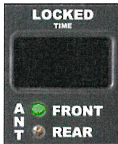
Figure 3.2.2.4b Antenna lights showing front antenna is active
