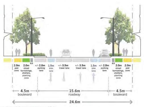
This cross-section represents the Larch Street extension west of Elgin through the Rail Lands. The existing function, character and right-of-way dimensions for Larch Street should be preserved east of Elgin Street.
