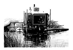
Dominion Divers Ltd.'s SUBCAT is a submersible self-propelled crawler operating on two 32-inch rubber tracks resulting in only .5 PSI ground pressure. This eliminates the danger of breaking the bottom seal of the containment area.
